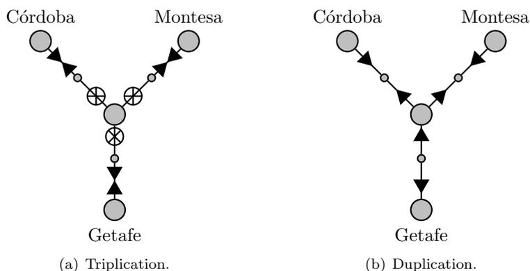
Figure 2: Y-shaped modeling of a compressor station.
